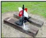
**SWITCH ALIGNMENT:** **White** or **Green:** Proceed - switch aligned
